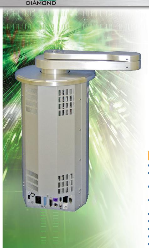
The Diamond H<sub>5</sub> series vacuum robots represent a significant engineering advancement in the design and reliability of wafer handling equipment.
