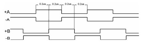
Encoder signal waveforms (CW direction)
