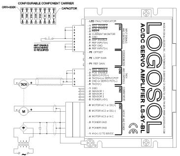
In this configuration the amplifier drives a motor-tachometer pair keeping constant speed. Motor speed is adjustable with **P3** OFFSET. **P1** REF GAIN has no effect if **REF INPUT (+)** and **REF INPUT (-)** are grounded, otherwise set P1 REF GAIN fully CCW. All remaining settings are the same as described for typical velocity mode application.
