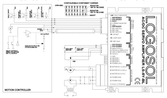
In analog position mode, an analog 10K potentiometer is mechanically coupled to the positioned object. The potentiometer supplies voltage proportional to its position. This voltage is used as a feedback signal, which drives the motor keeping the potentiometer position proportional to the reference input voltage.
