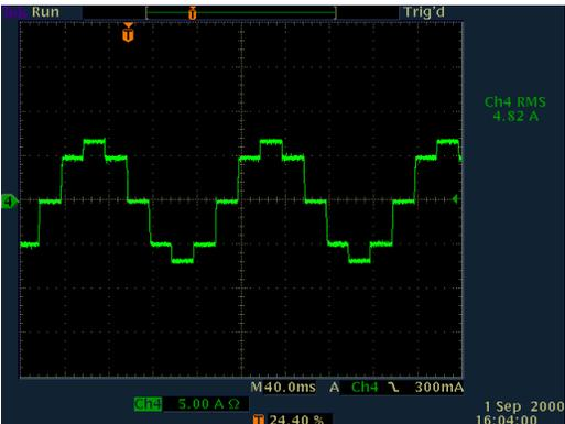
Winding current in half step mode with torque compensation
