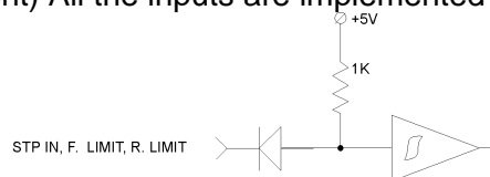
Limit Switches and Stop Input
